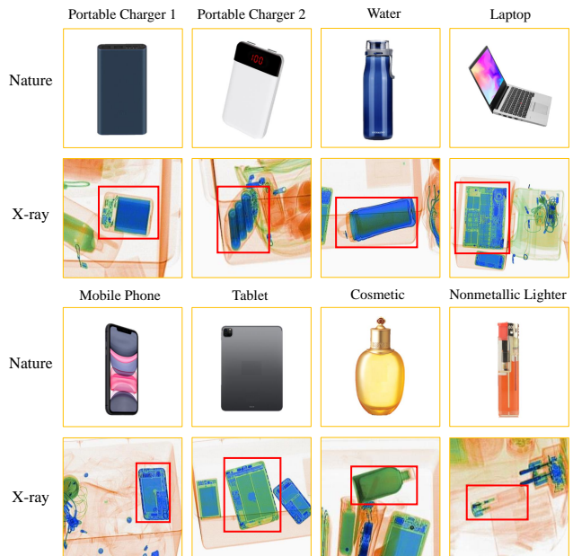
Figure 1. Nature and X-ray images of the 8 categories of common prohibited items in HiXray. These prohibited items usually contain lithium battery, liquid, lighter, etc.
